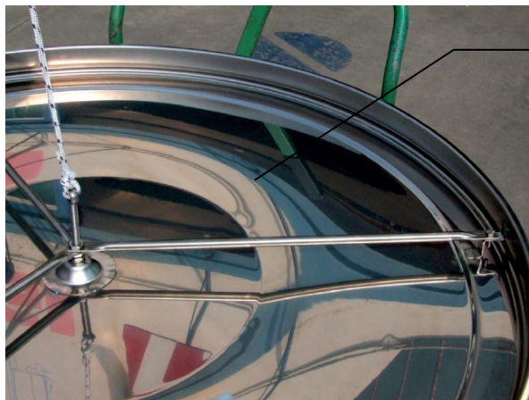
Figure 30: Assembly of floating tie rods.
